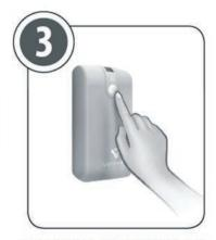
**TURNING THE DEVICE ON** When the wraps are secured on your legs PRESS and HOLD the WHITE power button for about a second until the light is illuminated on each unit.
